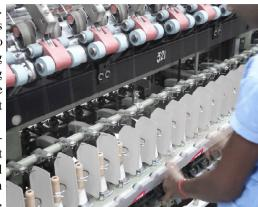
information to indicate the end of traveler life cycles. The bobbin built-up report allows the mill to monitor traveler wear related to "We invested in Uster age, checking stable end-break rates through the entire doff duration. Sentinel ring spinning This report shows the current state in intervals of five minutes, optimization system with the and an overview provides information about end-breaks per 1,000
